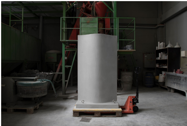
Fig. 4. IF building a mesh prototype. (b) Filled steel-reinforced wall prototype.
