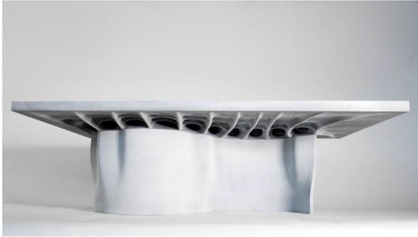
Fig. 20. 1:10 model of the final design: the ceiling rests on a linear beam, following the upper contour of the wall.
