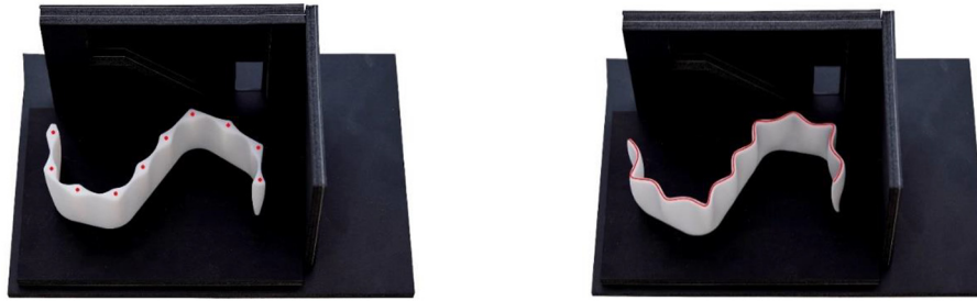
Fig. 19. Design examples for different structural scenarios: (a) local thickening of the wall as a reaction to concentrated loads; (b) local undulations as a reaction to linear loads.
